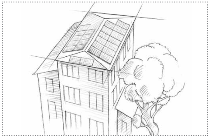
Multiple orientations, no problem: Installers can now use roof space on multiple sides of a home (for example, south/west or east/west) to generate power.
